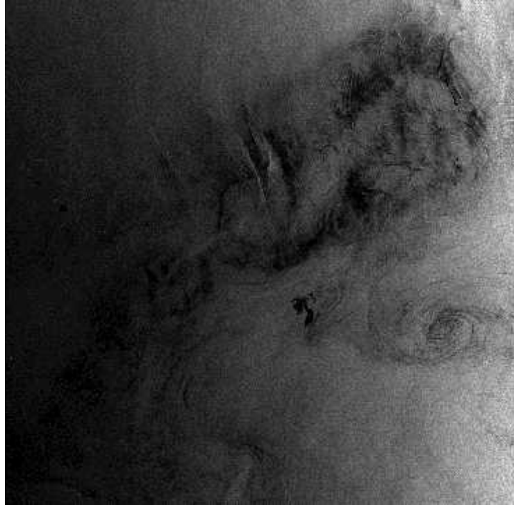
Figure 5. Envisat ASAR image of the open South-China Sea acquired on 13 March 2010 at 02:19 UTC showing spiral eddy 1, oil spill 2, arciform imprints of internal waves at the upper right, numerous filamentary slicks and ships (bright dots).
