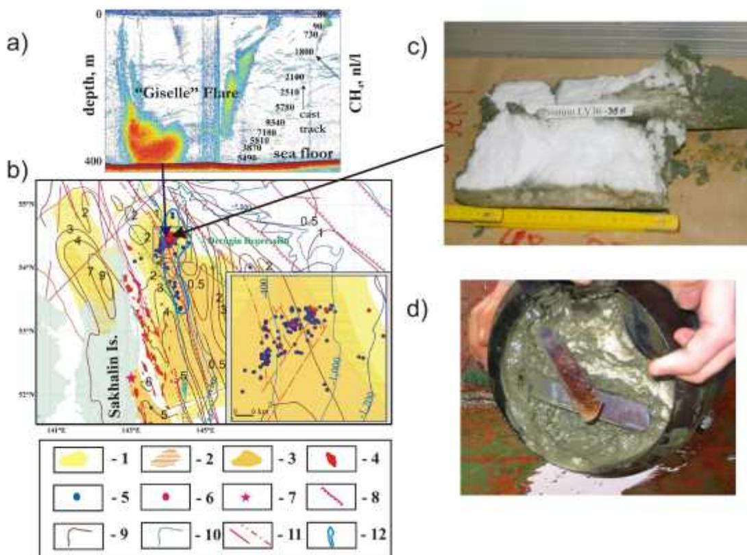
**Figure 11.** Gas hydrates in the Sea of Okhotsk (NE slope of Sakhalin Island). a – gas flare; b – geological structure of gashydrate cluster; c – piece of gashydrate; d – gas hydrate bearing sediment core.
