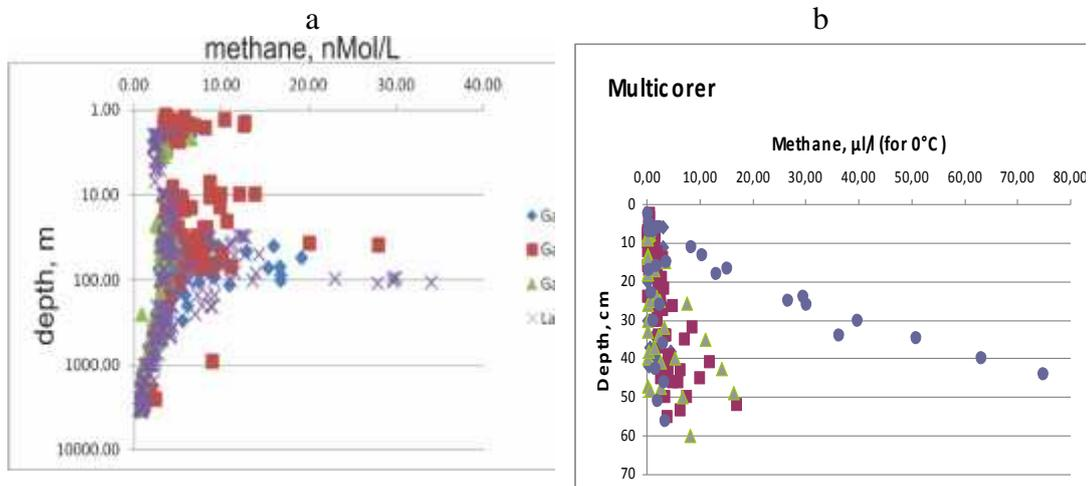
**Figure 3.** Common vertical profiles of methane in sea water (a) and sediments (b) of Japan Sea (nMol/L) for 2009-2010.. Distribution of CH<sub>4</sub> (nmol• L<sup>-1</sup>) in the subsurface sediments 5-60 cm (Vereshchagina et al., 2013). Profile D show the sharp increase of the methane concentrations within the fault structures.
