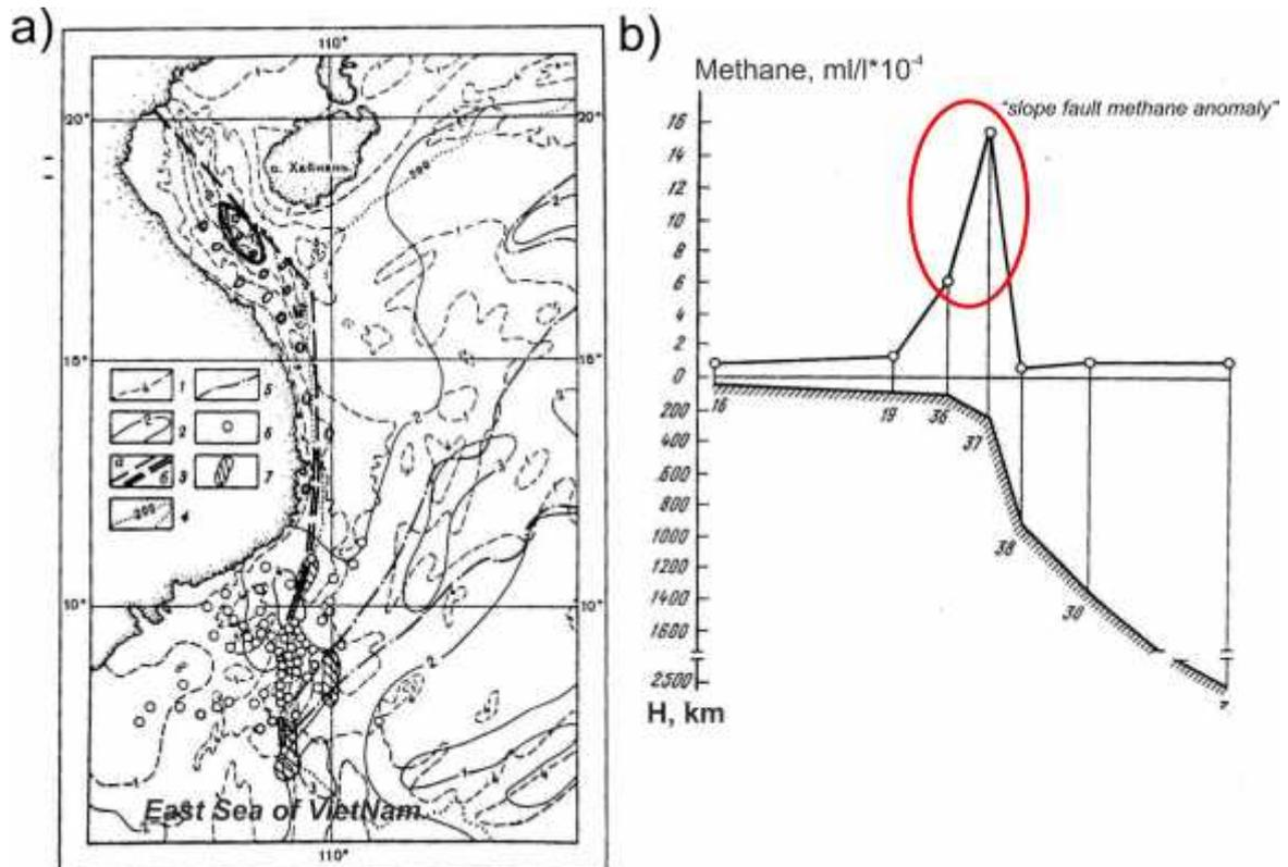
**Figure 14.** Scheme of gasgeochemical study in the East sea of VietNam during 1983;1989 (head of expeditions Prof. Anatoly Obzhirov). Map of gasgeochemical study on east sea of VietNam in 1989. a) 1 – acoustic basement; 2 – heat flux; 3 – faults; 4 – depth 200 m; 5 – sub-oceanic crust; 6 – gasgeochemical stations; 7 – ultra basic rocks (by geophysical data; b) – methane distribution across South-KonShon Basin (1989).
